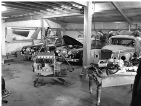
2 V8's, Majestic Major and Special Sport engine and gearbox in foreground.
