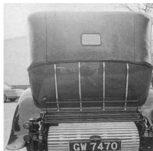
Familiar to many Daimler owners is the slatted protection across the fuel tank at the rear.
