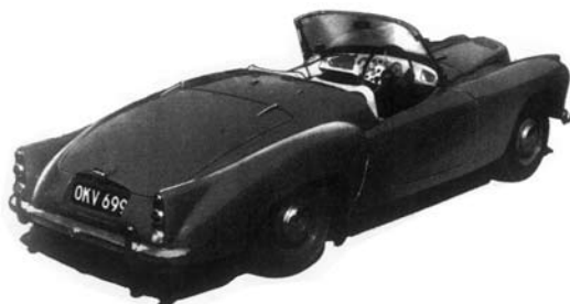
TWIN rear lamps, reversing lights and flashing direction indicators are built into a fin extending from the rear wings. The large expanse of the luggage boot lid is a noticeable feature of this view of the car.
