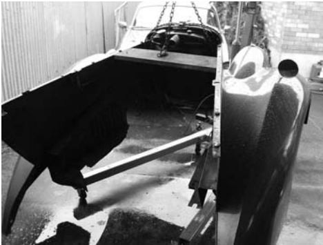
57. Front assembly removed.
