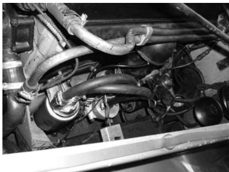
62. New engine installed. Note oil filter (left) is accessible from under bonnet.
