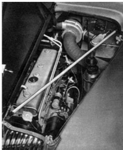
The coil and distributor are mounted on the left-hand side of the engine, with the dipstick between them. Most routine maintenance, including checking engine oil, radiator and screen wash bottle levels, can be done from this side; the right-hand side of the bonnet gives access to the brake fluid and one-shot lubrication reservoirs.
