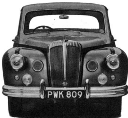
The familiar fluted radiator grille maintains the traditional appearance. Twin fog lamps are mounted near the over-riders. Circular grilles on each side of the radiator supply fresh air to the beater, and ventilation for the driver in hot weather. The front pair of jacking sockets can be seen below the bumpers outside the over-riders.
