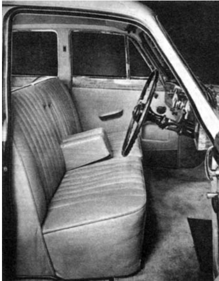
The interior of the Daimler is trimmed in leather and polished hardwood, with pile carpet. Pockets are provided in all the doors, and combined pulls and arm rests are fitted to the front pair. Folding picnic trays are built into the backs of the front seats.
