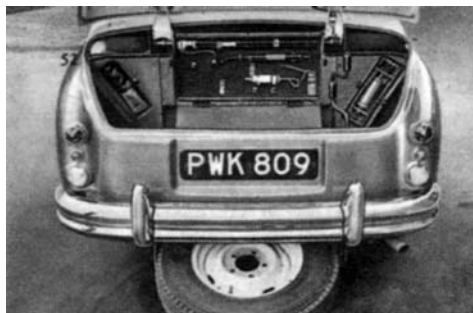
Three small lockers, built into the vertical wall of the luggage compartment, contain a comprehensive kit of tools, including a foot-operated tyre pump. The wheel brace and its extension are shown in use to lower the spare wheel tray.
