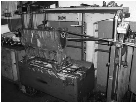
Block aligned and set up for line boring.
