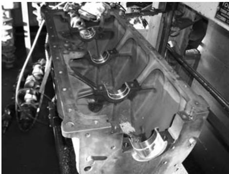
Main bearing in block after line boring.
