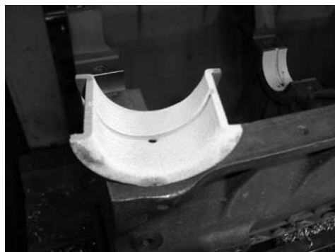
Main bearing shell after metal spraying.
