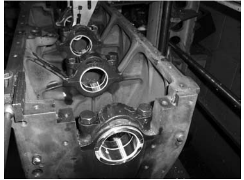
Main bearings after machining. Note thrust surface on No. 1 journal.
