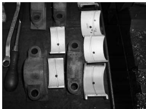
Main bearing shells after metal spraying.
