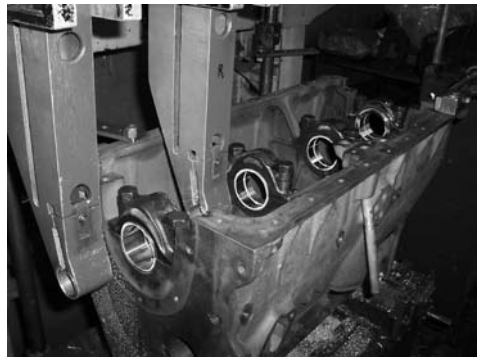
Main bearings after line boring.
